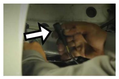
6. Remove Lower Strut Mounting Bolt.
