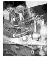
Nuts Front axle shaft Spring strut Wishbone
