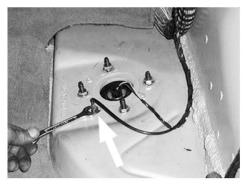
4. Disconnect the electrical connector from the top of the air strut (push on the sides of the connector to release.)
