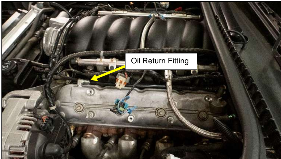
Driver's Side Valve Cover Installed
