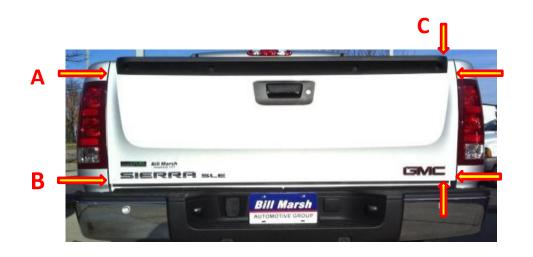
This sheet is to help eliminate any confusion about which gate the retail customer needs to order due to overlapping styles of OEM trucks at model change-over. Measure the *factory tailgate* at points A, B and C to confirm the proper fit for the customer's truck.
