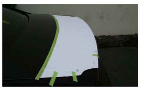
3. Tape template into position and center punch where marked. Drill holes to 11/32". Be careful at trunk rear.
