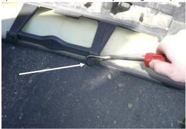
7. Cut off the four mounting tabs on impack bar as marked in photo below.
