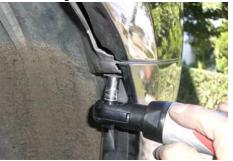
**3.** Located on the mounting lip of the OEM rear fascia to the rear of quarter panel are two retaining fasteners. Pry out the white center pin on these. DO NOT pry out all the way. Pry out a maxium 3/4".
