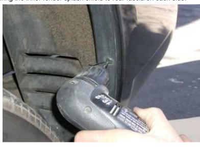
2. Using a 9/32 socket remove the single bolt on each side, securing the inner fender splash shield to body.
