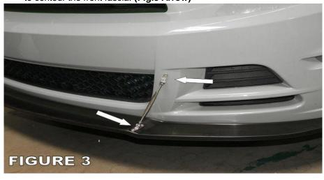
**5.** Last you will be installing the turnbuckles onto the front fascia and the top of the splitter. Use the provided small self tapping screws and mount as shown or any way you like. Now you are done. Enjoy you new look.
