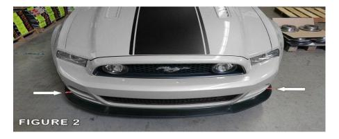
3. Next you will need to secure the end on the side of the splitter. Use the big self tapping screws and mount 2 on each end. It is recommended that you drill pilots holes in the locations you will be securing the splitter.
