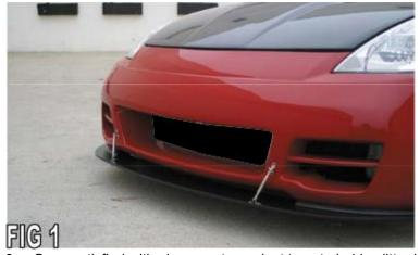
3. Once satisfied with placement use duct tape to hold splitter in place and drill holes for the M6 bolts through both splitter and fascia in 3 places on either side of the splitter opening. As shown in (Fig 2) as well as the center hole for the center support.
