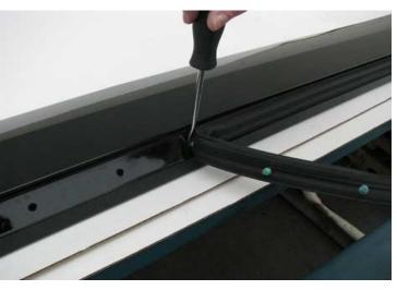
8. Next you need to open the door and get ready to install the door seal on to the Street Scene Side Skirt. You will see all of the holes in line. Drill out with a 3/16 drill bit, then you can install the door seal. See photo below.
