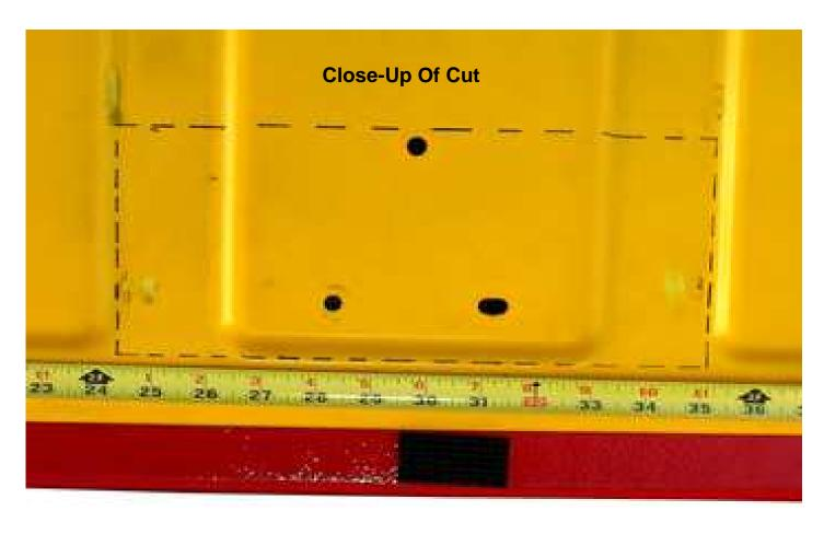
2. Measure down from the top edge of tailgate 2 1/2" and mark the 1st horizontal line. Make your next mark 4 1/2" down from the previcously marked top line. Double check your measurements. See Photo Below
