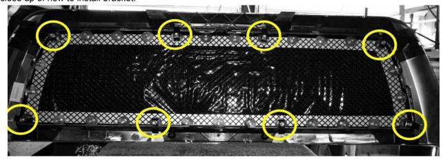
**5.** Place all 8 nuts and brackets in corresponding points before securing to shell. Do not over tighten.
