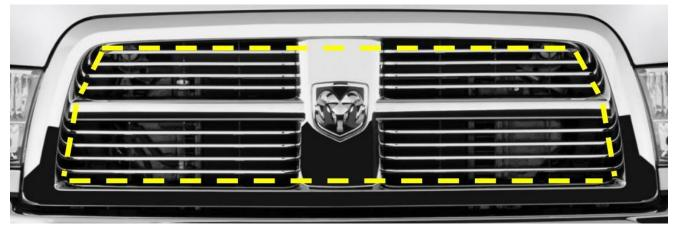
2. Leave a 1/4" lip on the four center cross bars. The new grille insert will rest on here.
