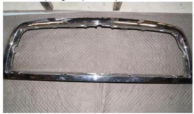
**4.** The longer bolts on the grille will be the ones used to install the brackets and nyloc nut. Step 5 shows a close up of how to install bracket.
