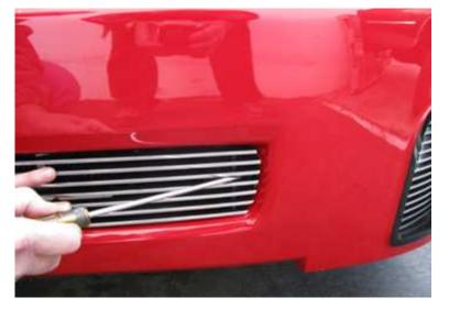
950-80198 BILLET GRILLE SET STREET SCENE BUMPER COVERS PART NUMBERS 950-70177 & 950-70198 **3.** Install the side billet grilles into the side openings. Drll an 1/8" hole through the mounting holes and into the bumper cover.
