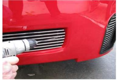
2. Install a phillips head screw into the bumper cover with the retainer nut placed on the back side.
