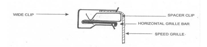
Push grille all the way in. Using the narrow attaching clip, attach the lower side of the "Speed Grille " at the center to the right and left of the " Bow Tie " and at each end one centered between.
