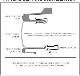
3. Attach the bottom side using the push in fasteners. Drill a 1/4" hole and push in to retain.
