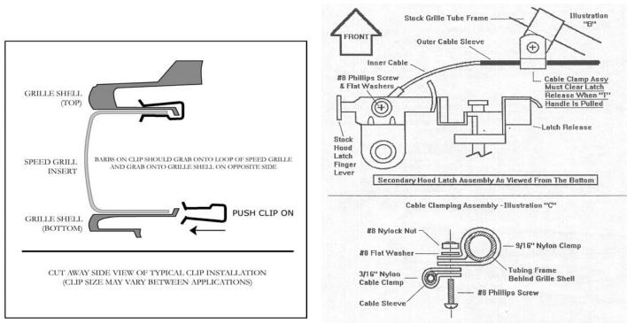
To assemble, first snap the clamps over the cable & tubing. Squeeze the clamps together to insert the #8 screw. Route cable, then tighten.
