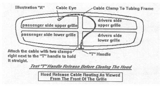
7. Install the Remote Hood latch Cable assembly starting with attaching the cable eye on the top side of the stock release lever hole. Fasten with a # 8 screw, ny-lock nut and flat washers provided. Place the flat washers on each side of the latch hole and tighten the screw just enough so the cable end can move back and forth for ease of operation.
