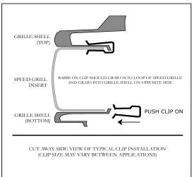
3. Install Grille Sheel back onto vehicle.
