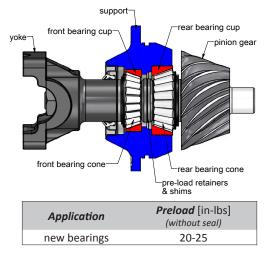
Bearing preload is the measure of torque [in-lbs] required to rotate the pinion after the nut has been torqued to spec.
