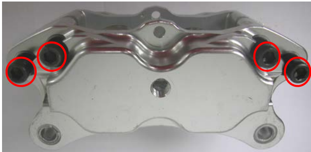
Figure 1: Four Caliper Bolts Removal
