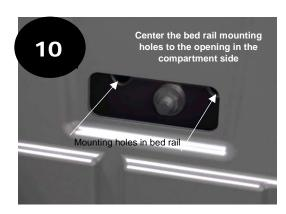
To locate the cargo compartment in the correct position relative to the truck box, first align the hinge mounting holes on the both sides of the compartment with the mounting points in the bed rails.
