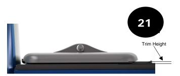
Re-position the striker vertically as required to adjust the trim height of the cover along the side of the truck while maintaining the latching function to the striker. The trim height should be even from front to rear looking at the cover side rail on the driver's side.
