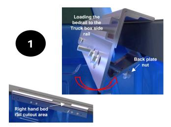
Loosen the back plate nuts to the end of the bolts and load the bed rail to the truck box.
