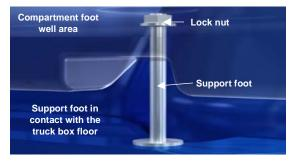
Loosen the lock nut and turn the support foot downward until it rests on the floor of the truck box. Retighten the lock nut to secure the support foot in place.
