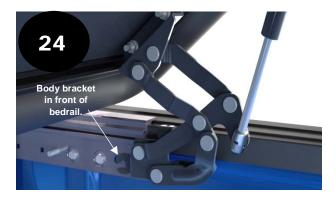
With the assistance of an associate lift the cover into position just behind the bed rails. Move the cover forward until the hinge body bracket starts to overlap the end of the bed rails.
