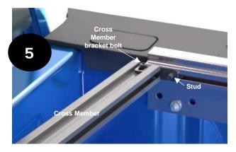
The cross member is installed from the front end of the bed rail at the truck box head board.
