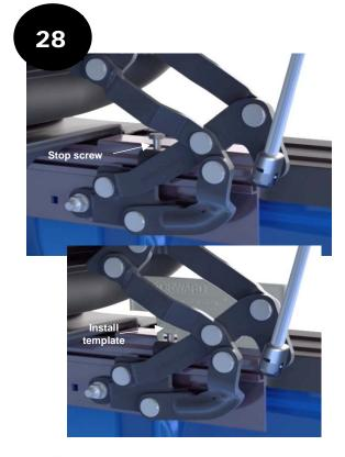
Install the rear hinge stop screw and set the installed height using the cutout in the bed rail installation template.
