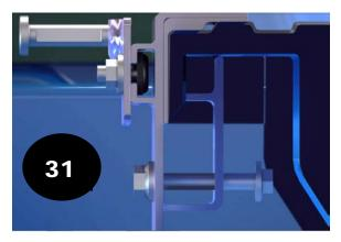
Secure the bed rail fasteners while holding the bed rail and back plate in position.
