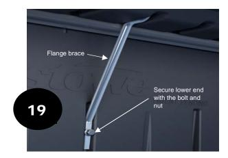
Install the cargo compartment rear flange brace by inserting the top end of the brace into the underside of the flange and placing the lower end of the brace against the front face of the cargo compartment.
