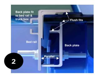
Raise the bed rail back plates until flush with the underside of the truck box while keeping it parallel to the back side of the bed rail.
