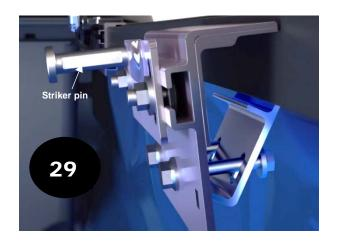
The rear bed rails are unique to the left and right side of the truck. Ensure that the striker pin is positioned towards the rear.
