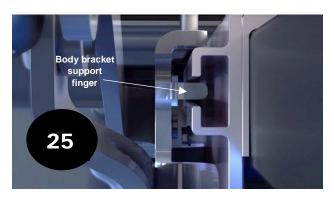
Move the panel forward and insert the body bracket support finger into the channel on each bed rail.
