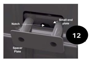
Install the hinge mounting spacers through the compartment wall opening. Accomplish this by tipping and inserting the lower edge of the smaller end plate into the opening and then rotating the plate through the opening. The notch in the smaller end plate must face downward.
