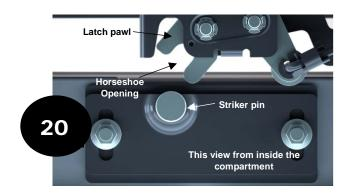
Inspect the relationship between latch pawl and the striker as the cover approaches the closed position. The horse shoe shaped opening in the latch pawl should be centered around the striker pin.
