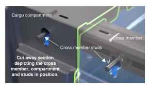
Lift the rear of the compartment upward to allow the cross member to be slid into the channel on the underside of the flange.
