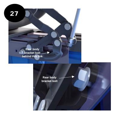
Install the rear body bracket bolts. Slide the bolt upwards through the slot in the body bracket until aligned with the bed rail nut and tighten.
