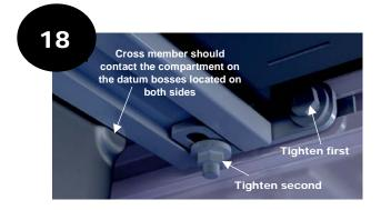
Tightening the striker nuts will firmly seat the cross member against the rear of the cargo compartment.
