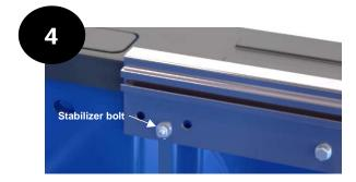
Loosen the jam nut and thread the stabilizer bolt through the bedrail until it firmly contacts the truck sheet metal behind the bedrail.
