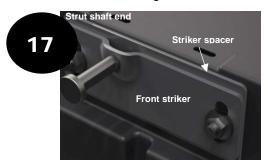
Install the front striker spacer through the rear of the compartment over the exposed cross member studs. Load the front striker to the spacer and hand start the stud nuts.
