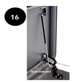
Install the struts by snapping the strut socket over the ball studs on the hinge and cover. Install the hinge end first.
