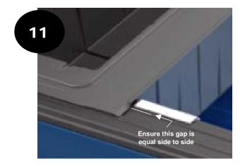
Then ensure that the compartment is positioned evenly side to side by inspecting the relationship between the rear flange and the bed rail on top of the truck box rail.
