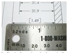
2. Check dimensions both vertically and horizontally to confirm it has been printed to scale.
