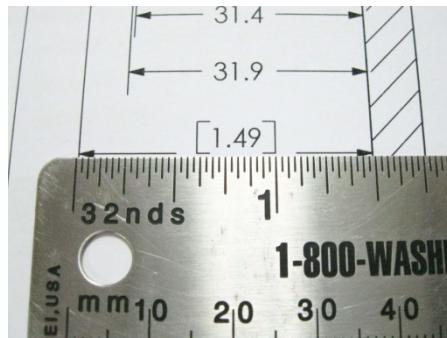
2. Check dimensions both vertically and horizontally to confirm it has been printed to scale.
