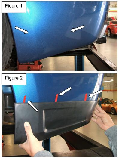
(**Fig.2**) Place the rear corner GENTLY on the vehicle and make sure you have it positioned correctly. If adhesion promoter was used you will NOT get a second chance! While holding it in position, pull the tabs you created while applying light downward pressure. Continue this taking care not to tear off the tabs by pulling to hard. After all the film is removed, apply firm pressure all around to insure the tape has bonded properly.
