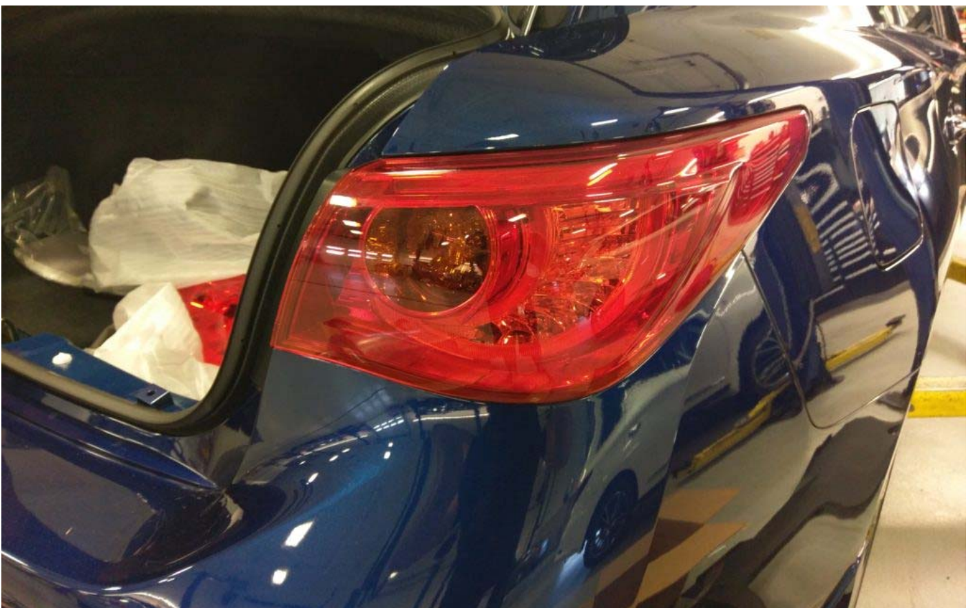
The Japanese Domestic Market (JDM) Q50 taillights feature an amber colored turn signal.
