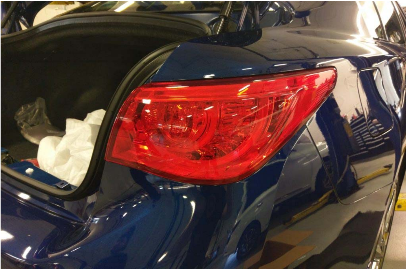
The US Domestic Market (USDM) Q50 V37 taillights are red on red, including the turn signal.
