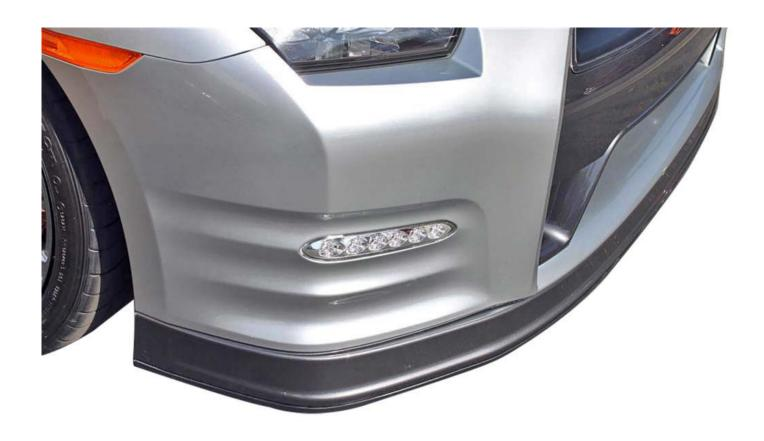
STILLEN has developed a urethane Skid Plate which protects the OEM fascia and paint from scrapes and light bumps. Durable urethane construction ensures no cracking, and doesn't require painting, although can be color matched if desired.
