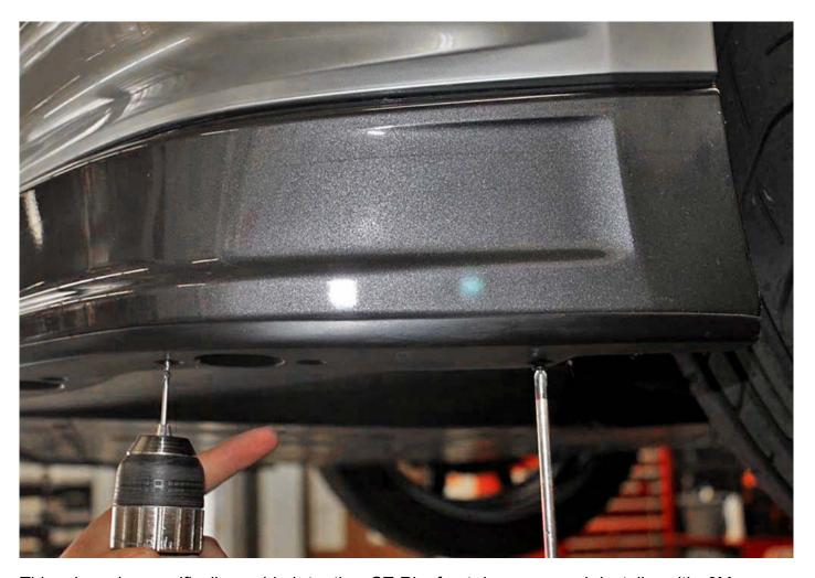
This piece is specifically molded to the GT-R's front bumper, and installs with 3M automotive acrylic foam tape and self-tapping screws to the underside.
