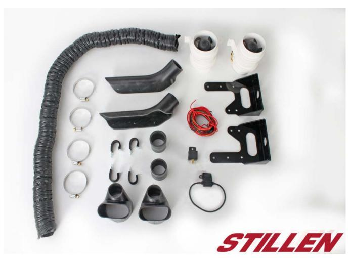
After months of testing and road racing, STILLEN is proud to announce the availability of the first Active Brake Cooling Package made specifically for the R35 Nissan GT-R.
