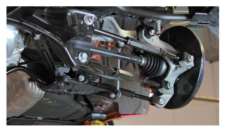
To make sure that the alignment was correct after the coil over installation and subsequent ride height lowering, SPC suspension provided a complete set of adjustable suspension including front upper control arms and SPC Suspension
