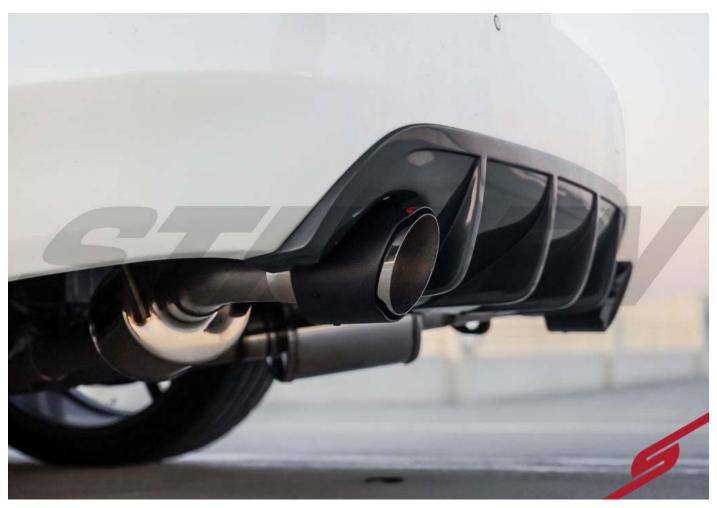
It's no secret that turbocharged engines thrive when allowed to breathe. Naturally-aspirated engines rely on some back pressure to create a scavenging effect to help maintain exhaust gas velocity. By contrast, turbocharged engines and particularly, the turbocharger(s), function most efficiently when the exhaust offers the least amount of possible resistance.
