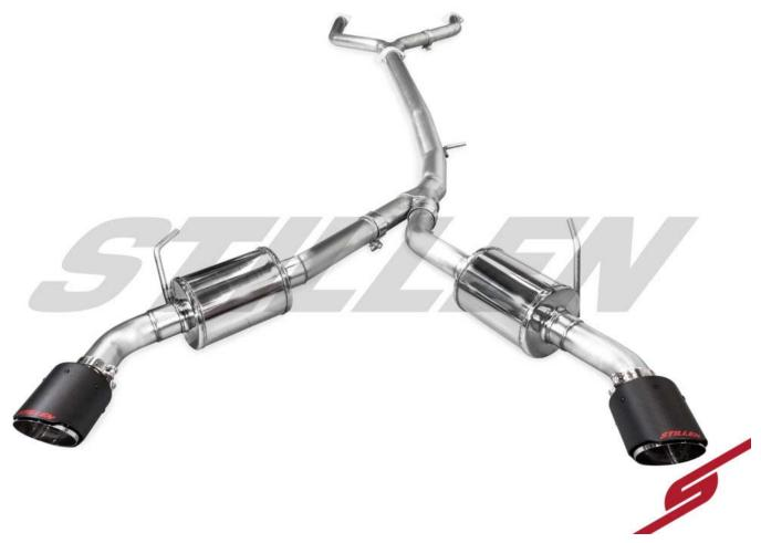
In the quest for the greatest gains possible, STILLEN engineers worked tirelessly to optimize this exhaust system. After several design revisions and numerous prototypes, this Cat-back Exhaust improved output with a best incremental gain of 21.37 horsepower at 4,750RPM and 23.94 lb-ft torque at 4,780RPM.
