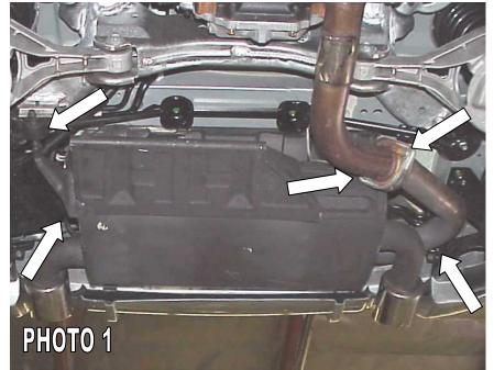
flange in front of the OEM resonator and pulling it out of the rubber isolator.
