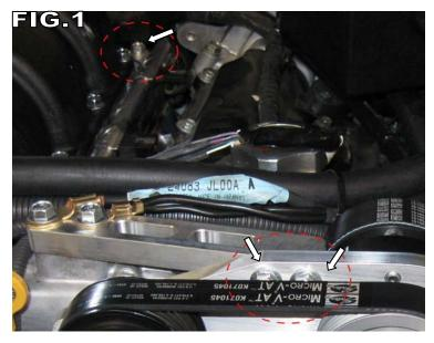
You will be installing the engine cover brackets where shown in (Fig.1) The taller one will go on the rear fuel rail bolt and the shorter one will be installed on the front 2 bolts which are holding on the support brace. See (Fig.2) You will be reusing the existing bolts already in place. For the front bracket it is recommended to loosen the bolts which secure the grounds onto the drive plate support.
