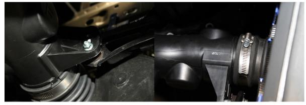
11. Remove the rear air box and air inlet assembly.
