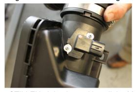
13. Install the MAF sensor into the STILLEN air intake and install the M4  $\times$  0.7  $\times$  12mm machine screws, M4 washers to secure the sensor. Torque the screws to 0.7 ft-lbs.
