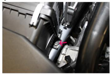
5. Remove the two nuts retaining the air box bracket (# 9 in the drawing below) and air box assembly as well as the nut connecting the bracket to the air box then remove the bracket.
