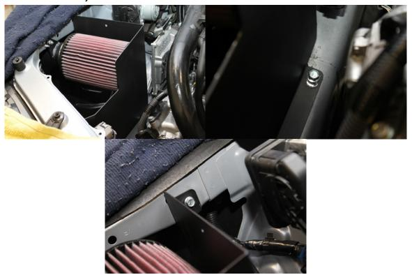
18. Reinstall the factory inlet scoop and adjust the heat shield to align the cutout with the inlet scoop. Tighten the two bolts for the heat shield.
