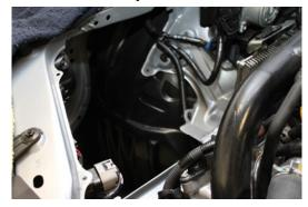
12. Remove the two screws retaining the MAF sensor from the factory air box and remove the sensor. Be sure to avoid touching the sensor element or hitting the sensor as it is very delicate.
