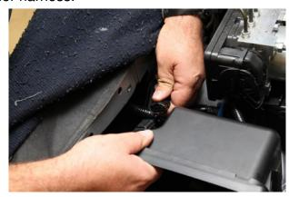
9. Remove the eight plastic retainers and one screw from the passenger side fender liner.
