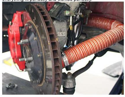
STILLEN Z34 Nissan 370z brake cooling kit installed
