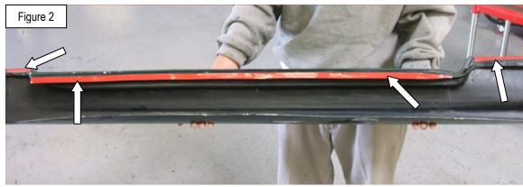
use of an adhesion promoter such as 3M <sup>™</sup> part #06396 should be applied to wherever tape will be used. When applying tape, make sure that tape is smooth and wrinkle free.
