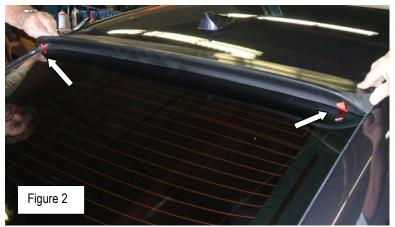
GENTLY on the vehicle and make sure you have it positioned correctly. It is a good to have a friend help with this. If adhesion promoter was used you will NOT get a second chance! While holding it in position, pull the tabs you created while applying light downward pressure. (**Fig.2**) Continue this taking care not to tear off the tabs by pulling to hard. After all the film is removed, apply firm pressure all around to insure the tape has bonded properly.
