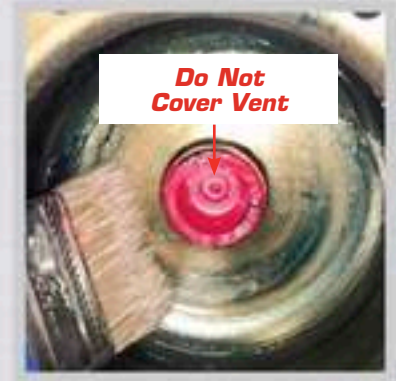
Fig. 3: Paint in the inside of stamped steel hub cap will grease
