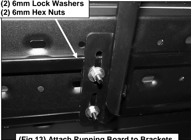
(Fig 13) Attach Running Board to Brackets
