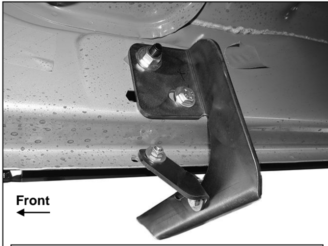
(Fig 15) Passenger/right Front Bracket installed (2013-on with factory holes pictured without Running Board for instruction purposes only)
