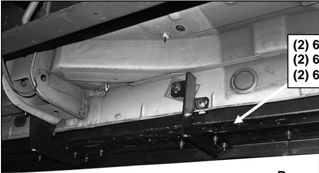
(Fig 30) Assemble Insert Tool as pictured. Turn wrench clockwise to pull/expand insert in hole
