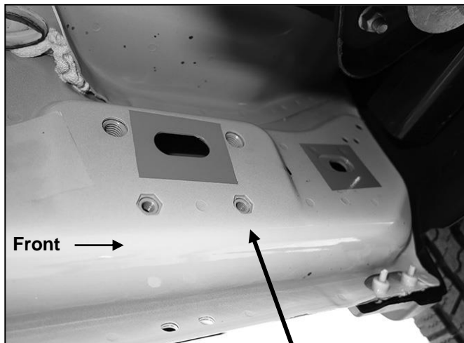
(Fig 4) Driver side front mid 2015-on and example of all models with factory installed threaded inserts
