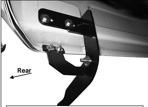
(Fig 16) Driver/Left rear Brackets installed
