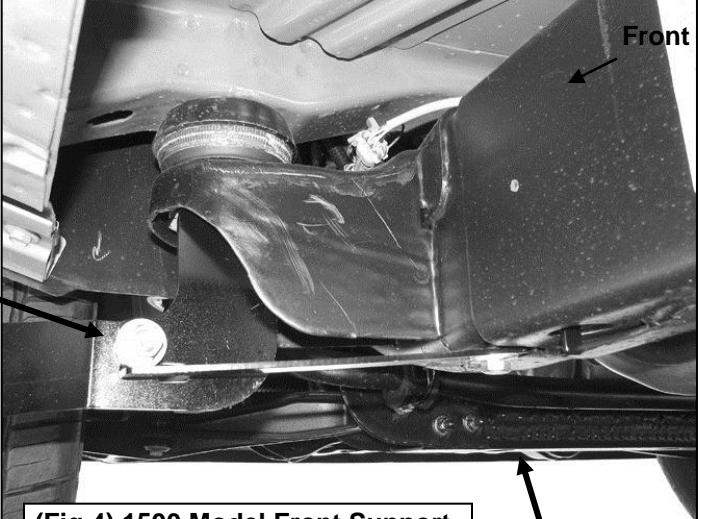
(Fig 4) 1500 Model Front Support Bracket Installation Pictured
