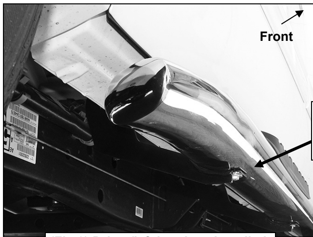
(Fig 8) Driver/left brackets installed
