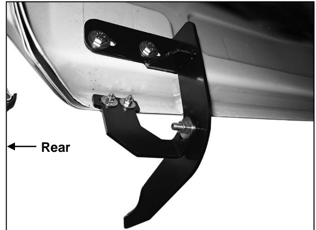
(Fig 18) Driver/Left rear Mounting Bracket assembly
