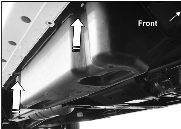
(Fig 12) Passenger side DEF tank and cover. Remove (2) hex bolts to remove straps for tank
