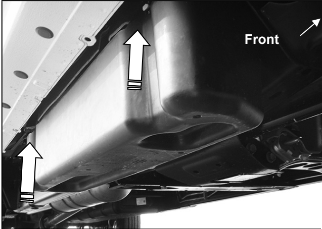
(Fig 12) Passenger side DEF tank and cover. Remove (2) hex bolts to remove straps for tank
