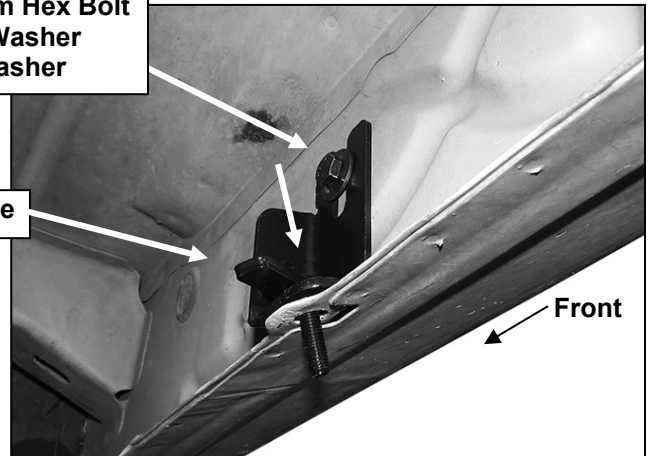
(Fig 16) On models with flat tab (see Fig. 3 & 4), insert 8mm Bolt Plate down through Upper Bracket and mounting tab
