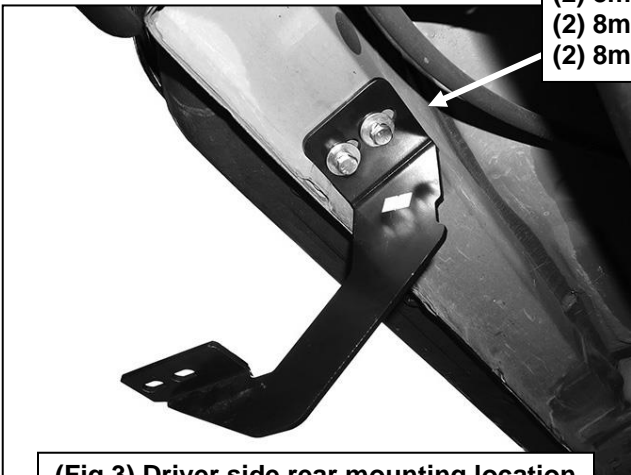
(Fig 3) Driver side rear mounting location
