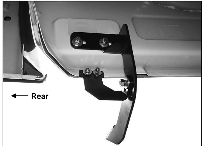
(Fig 16) Driver/Left rear Mounting Bracket assembly
