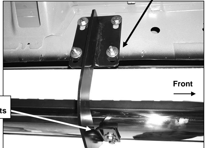
(Fig 7) Driver/left front Bracket installation pictured
