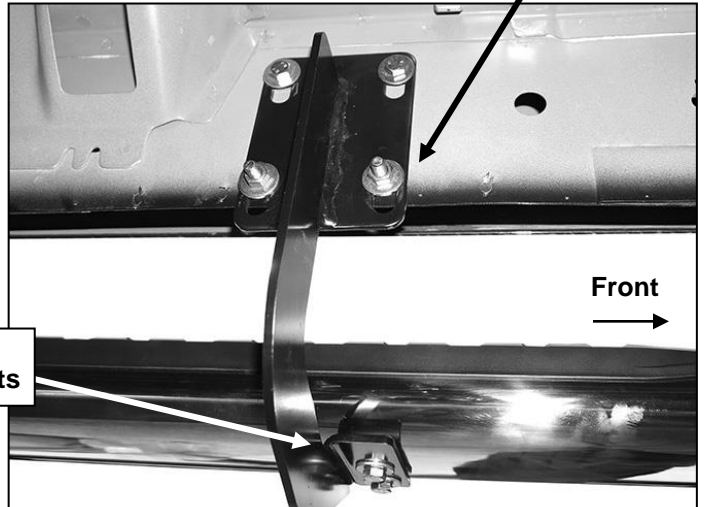
(Fig 7) Driver/left front Bracket installation pictured
